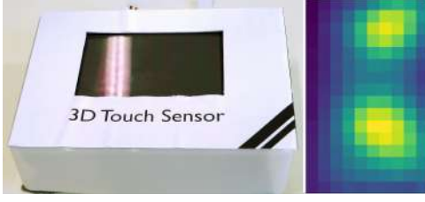
Figure 3: Left: The 3D sensing device, which also has a built-in display. Right: Raw output of the 10x16 sensor with two fingers hovering at approximately 0.5cm.
