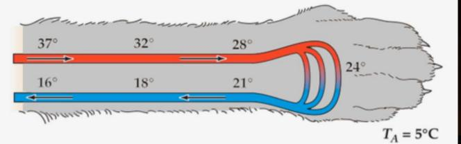
(b) Blood flow with countercurrent heat exchange
