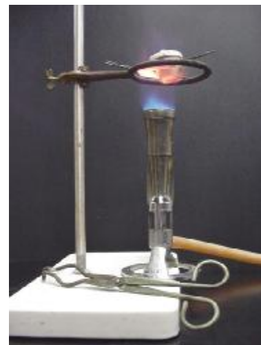
Figure 1: Set-up for heating a crucible. web.centre.edu/che/che131_lab/Exp3crucible.jpg
