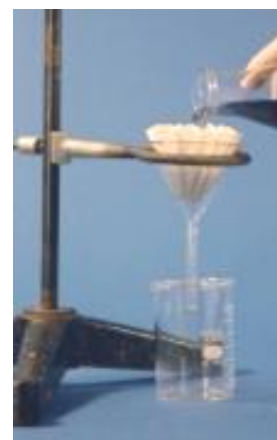
Figure 1: Gravity filtration set-up http://www.chem.ucalgary.ca/courses/351/laboratory/filtsmall.jpg
